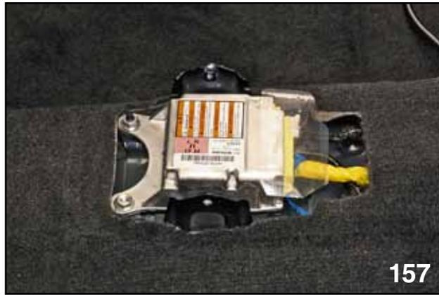
*SRS CONTROL UNIT BETWEEN REAR MOUNTING POINTS OF CENTER CONSOLE*
