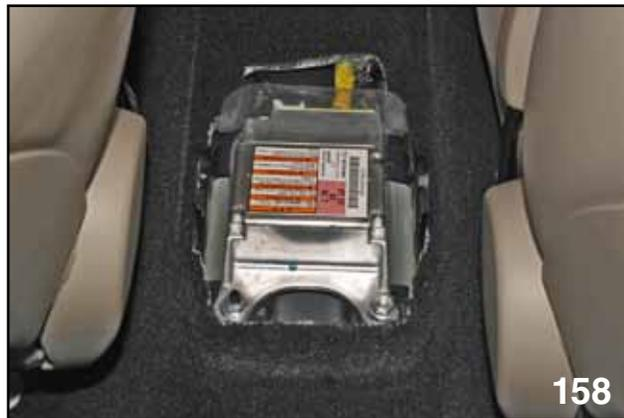
*SRS CONTROL UNIT MOUNTED REAR VIEW*
