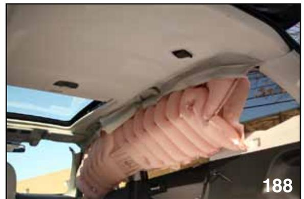
*HEADLINER AFTER CURTAIN AIRBAG DEPLOYED*
