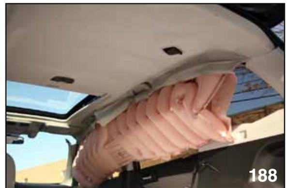
*HEADLINER AFTER CURTAIN AIRBAG DEPLOYED*
