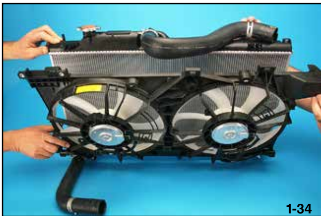
Removing Cooling Fans
