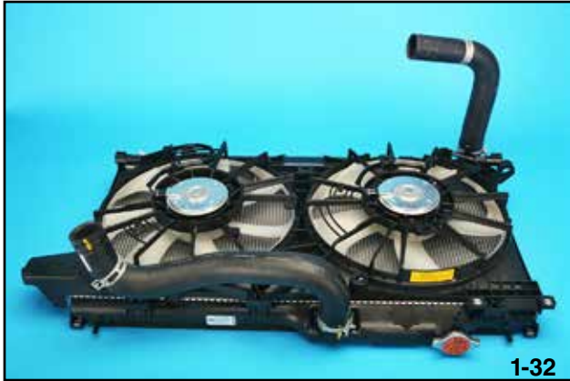
Radiator and Cooling Fans
