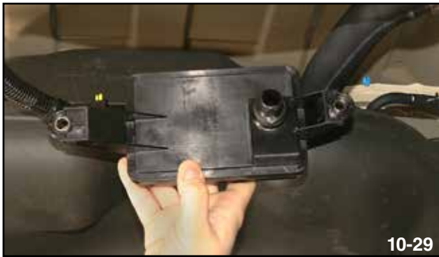
Drain Separator Removed
