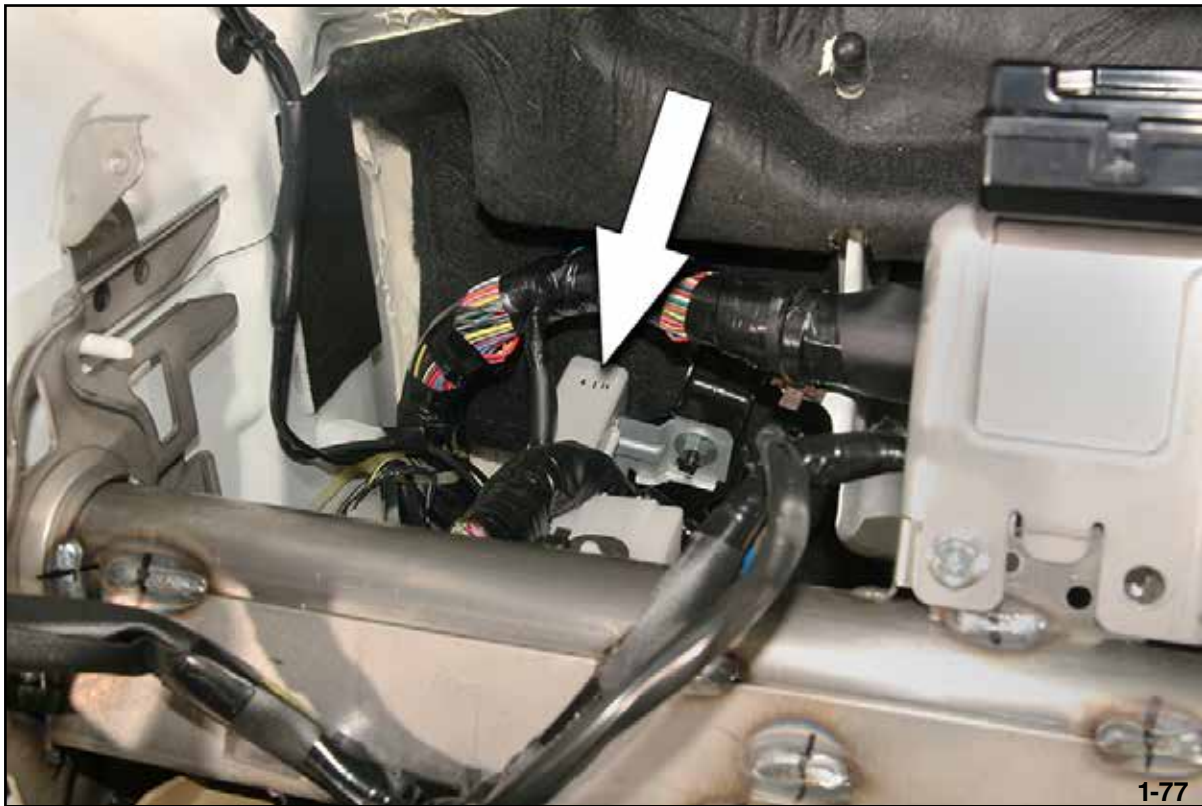
Left of Steering Wheel, Dash Pad Removed and Steering-Responsive Fog Light Control Unit (SRF)
