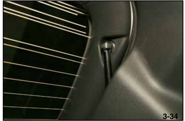
Top of Gate Lift Arm Gate Closed
