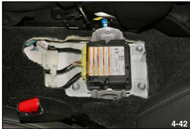
SRS Control Unit
