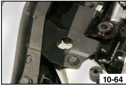
Radiator Garnish Opening
