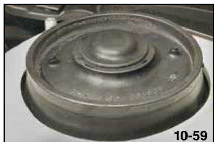
Rubber Strut Cap Installed
