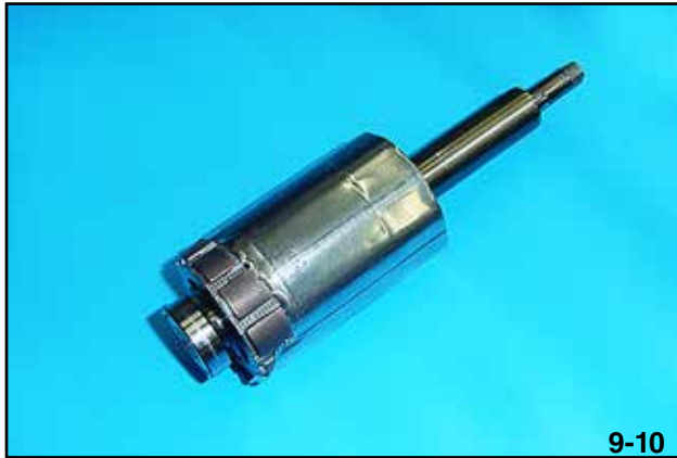
Exposed Rotor Magnets
