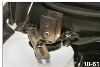
Lateral Bar Supports Installed
