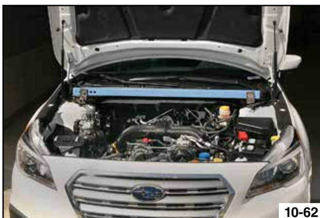
Lateral Bar Installed
