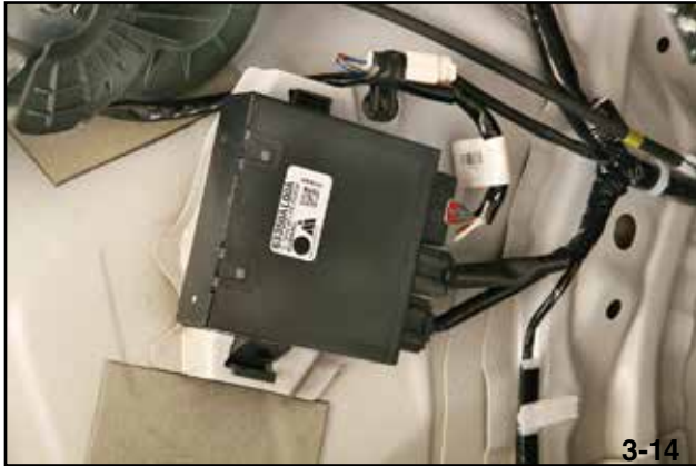
PRG Control Unit
