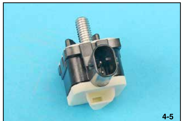
Front Door Sensor
