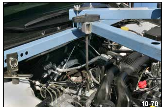
Rear Lifting Hook Installed
