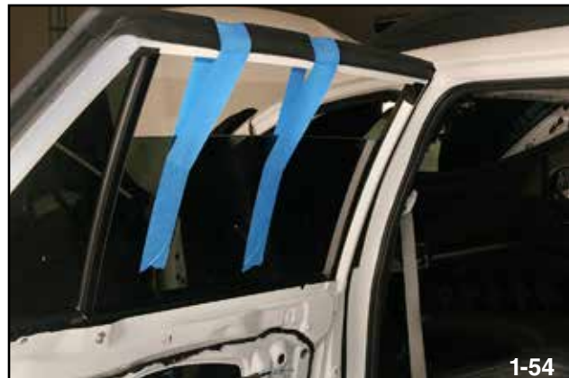
Window Taped In Position
