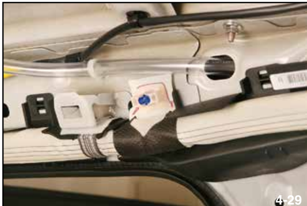
Installing New Clip
