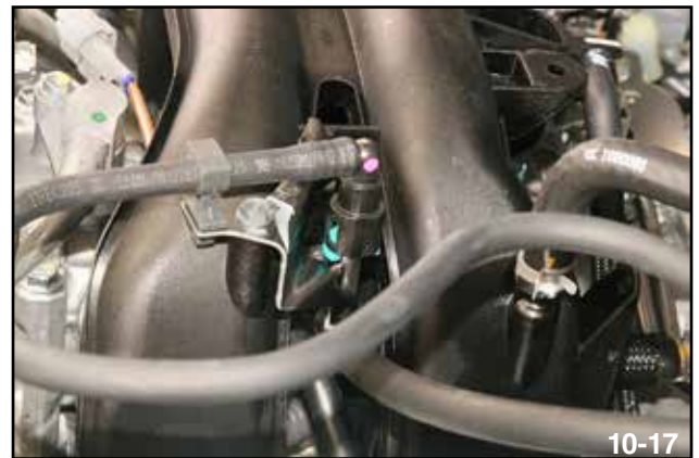
Fuel Line Connection
