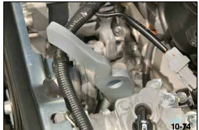
Front Hanger Installed
