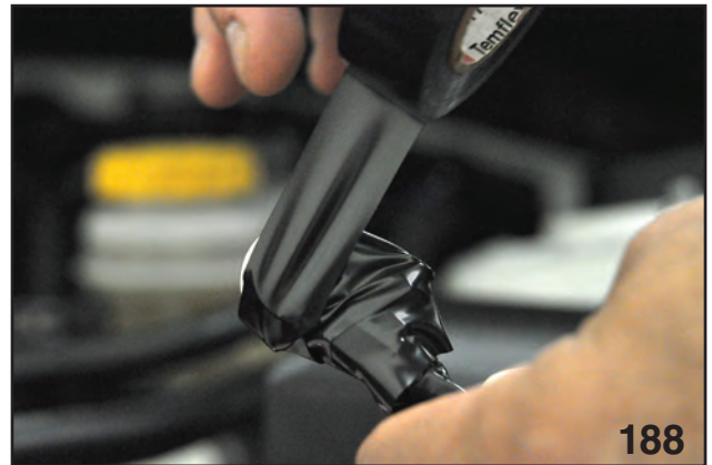
Auxiliary Battery Terminal
