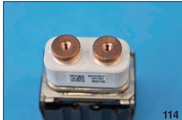
Contactor Connection Points
