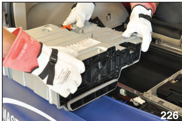
Removing High Voltage Battery
