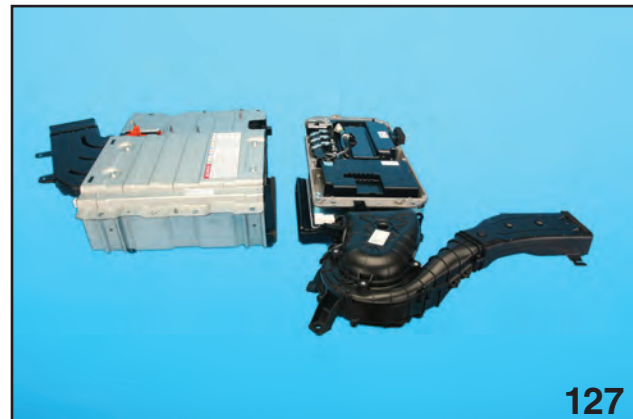
High Voltage Battery and Cooling System
