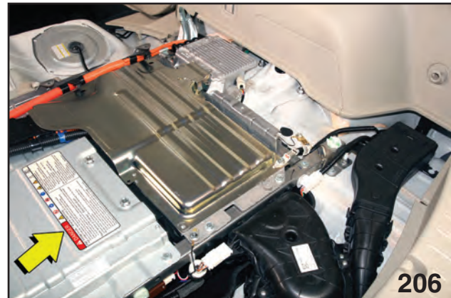
High Voltage Battery
