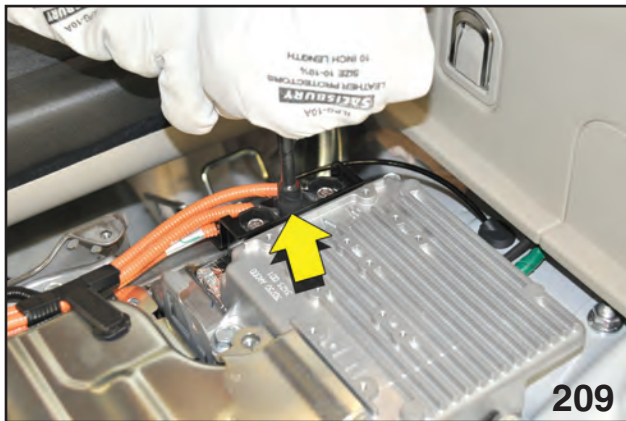
Removing Electric Oil Pump Wires
