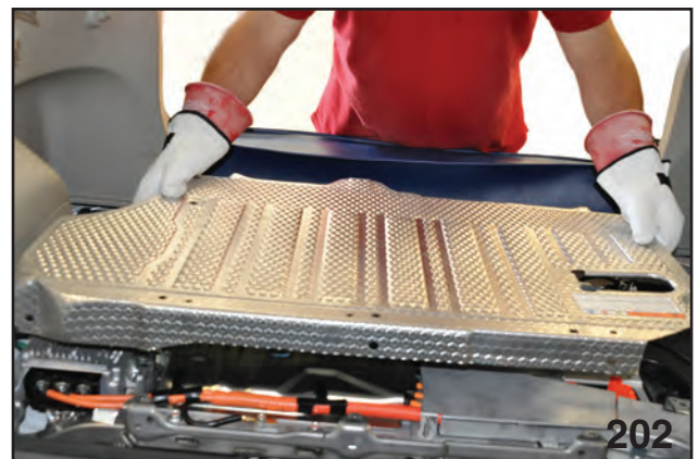
Removing High Voltage Battery Cover
