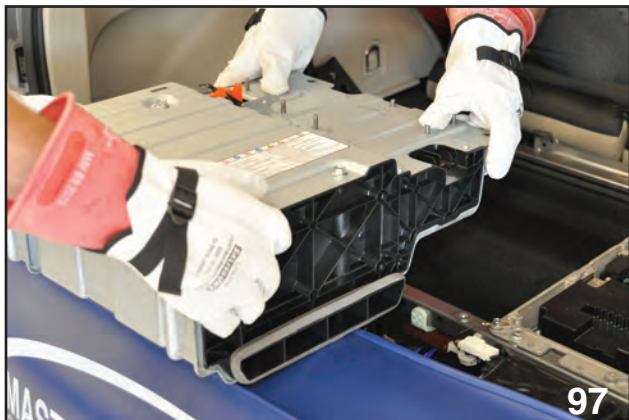
High Voltage Battery Removal
