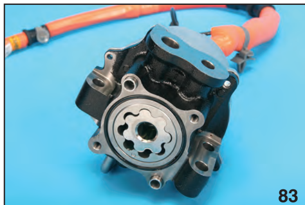
Internal View of Electric Oil Pump
