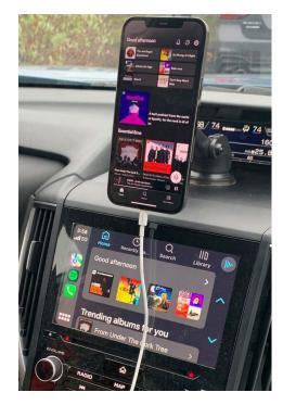
Finally, with the addition of CP1 to the Subaru lineup, there is a much larger screen where multiple inputs can be made. Shown to the right is an example of how a charging cord could affect the screen. This is especially noticeable in radio mode or a screen with several selections such as SXM or Navigation. This could cause a no response situation or screen distortion until the key is cycled and the cord is removed.
