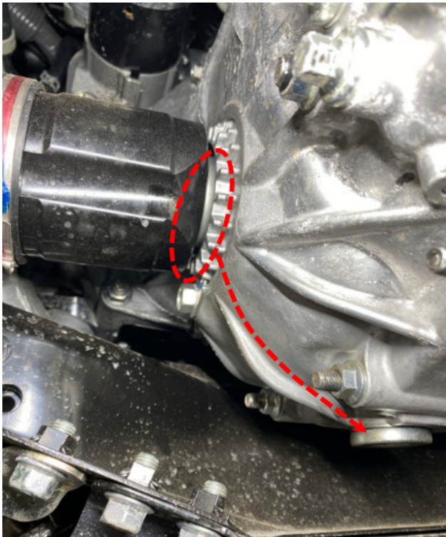
Fig.1 Junction of Transmission and CV drive shaft
