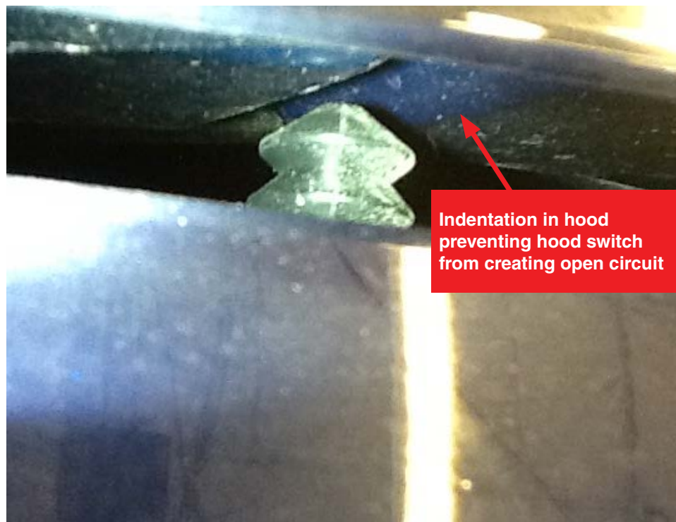
Figure 2 – Hood Switch Position Installed Incorrectly
