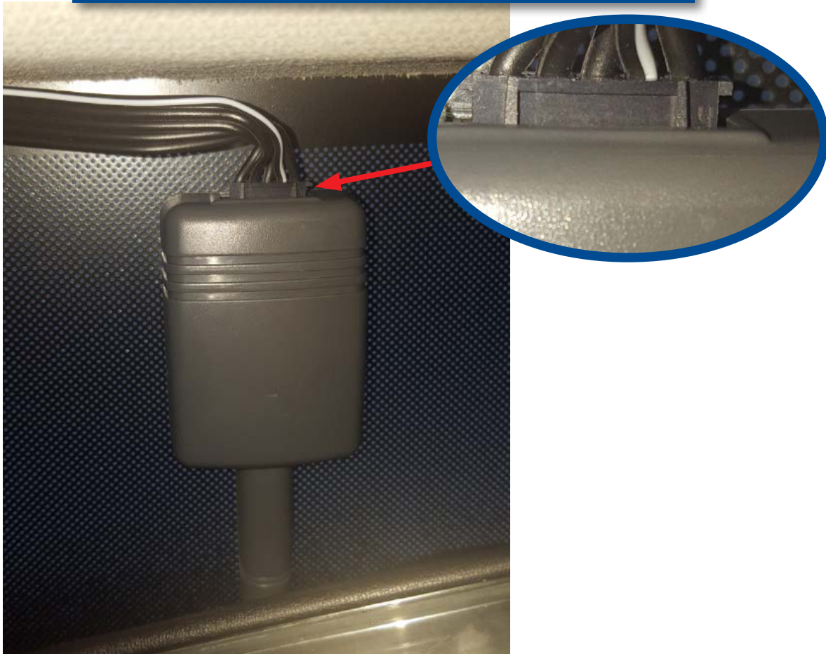
RES Antenna Connection – Secured
