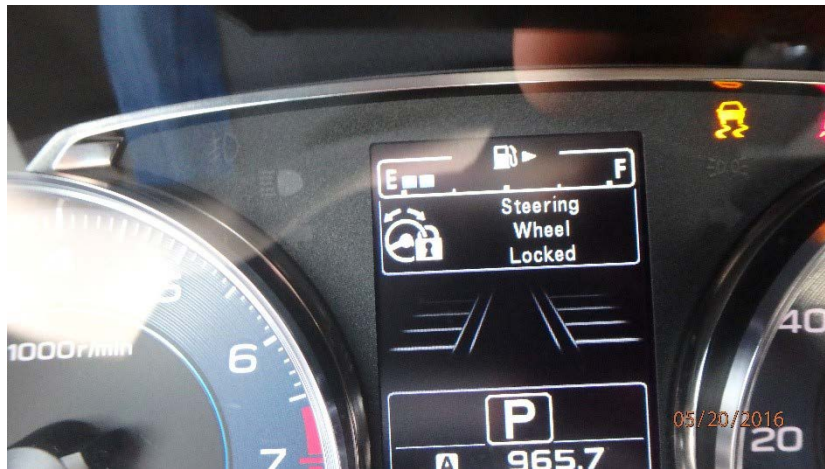
Steering wheel locked message in IP (Start button LED flashes GREEN)
