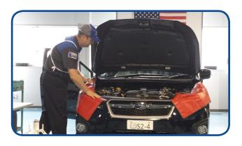
area. Experienced Technicians recognized the pitch and frequency of the noise as a valve related noise. Skillful use of the stethoscope narrowed the location to a #3 exhaust valve. This discovery resulted in the need to remove the corresponding valve cover and perform related valve clearance measurements. As with the Driveability event, Larson demonstrated expert skills in engine diagnosis, disassembly, precision measurement, and outright speed.
