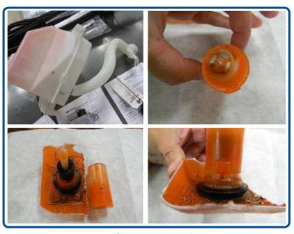
proper operation of the sending unit float and switch components. Some photos of the collected parts with the residue are shown on the right. This type of damage is to be considered resultant from an outside influence and therefore not a matter for warranty.
