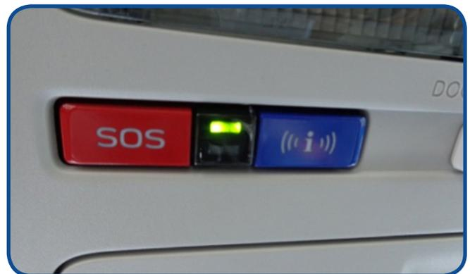
Figure 2) This condition indicates either Initial Activation is incomplete or the vehicle has an Active Subscription.
