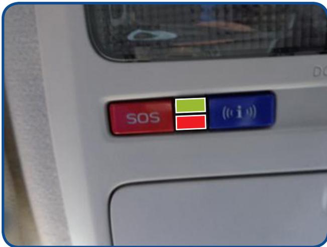
Figure 3) If both lamps are illuminated, this indicates the Telematics device is having a communications concern.
