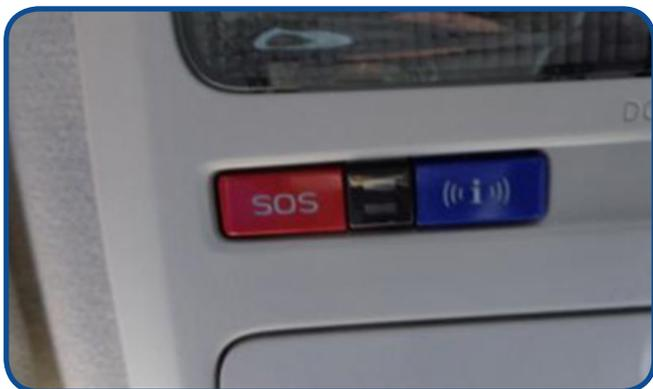
Figure 1) Both Telematics lamps are extinguished. This is the expected condition at PDI.
