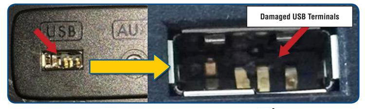
An easy way to prevent this type of damage is to make sure the USB icon which is usually found on the body of the device connector always points upward. The USB connector inside the console box can be difficult to see, especially at night. In that case, make sure the USB icon faces toward the molded-in "USB" when connecting the device. Never force any device when connecting or disconnecting it to or from the USB port.
