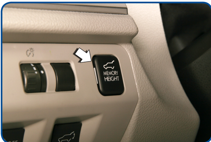
Memory Height Switch Highest Setting (OFF)
