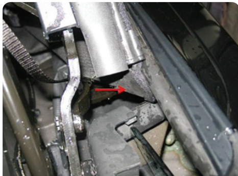
Correct position of the plastic water diverter
