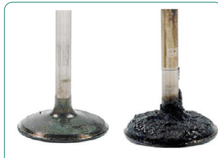
Intake valve (right) using gasoline with the legal minimum additive.
