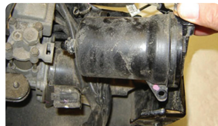
For sensor replacement, install a complete air filter, dryer, and sensor assembly.
