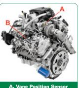
B. Electrical connector/module is available that interfaces with the ECM more efficiently.
