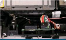
If a DTC P0AF8 or P0AFB is setting, the connections at the BECM, contactor relay and disconnect switch should be checked.
