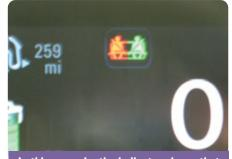
In this example, the indicator shows that the right-side seat belt is buckled and the left-side seat belt is unbuckled.
