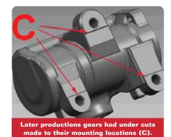
All production vehicles should have either the shimmed or the undercut mounting tab. If the steering gear is replaced in service, it is important to use the shim only when required.
