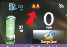
The rear seat belt indicator is in the center of the instrument cluster.
