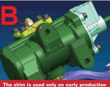
The shim is used only on early production gears that do not have the under cuts (B).
