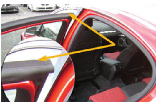
Location of water leak on the rear door
