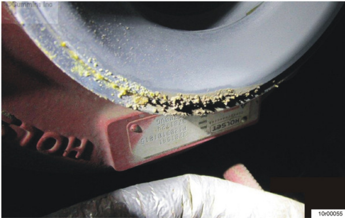
Figure 3: Buildup of dirt and debris on turbocharger compressor inlet.
