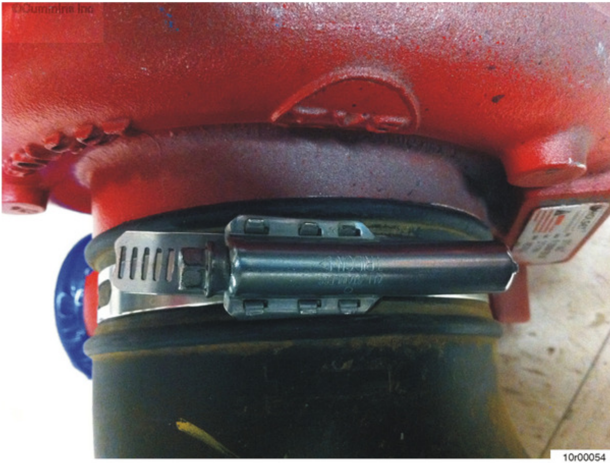
Figure 2: No gap present when clamp is at proper torque.
