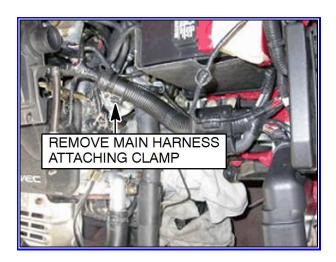
intake duct, air cleaner box and intake tube.4. Remove the main harness attaching clamp.
