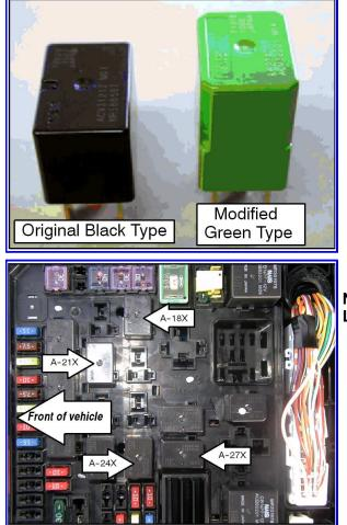
5. If no DTCs are reset, perform the following steps to replace the relays.
