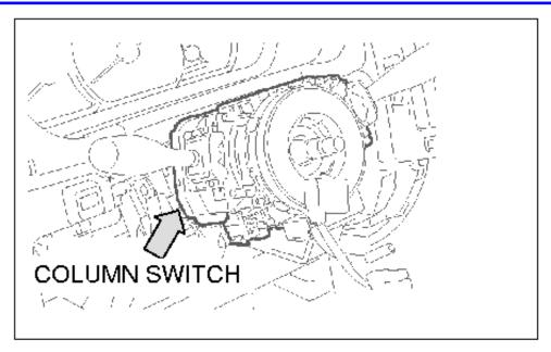
2.Remove the steering wheel assembly. Refer to Group 37 in the appropriate service manual. Then remove the column switch assembly. Refer to Group 54 in the appropriate service manual.
