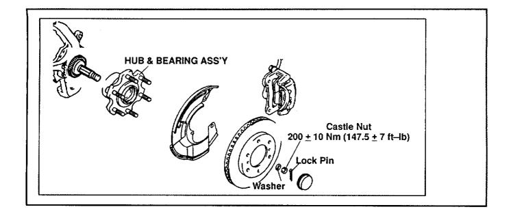
When installing the new hub assembly, make sure the castle nut is tightened to the new torque value (200  $\pm$  10 Nm [147.5  $\pm$  7 ft-lb]). The new-style castle nut is modified with a friction coefficient stabilizer and has a green color on its surface.
