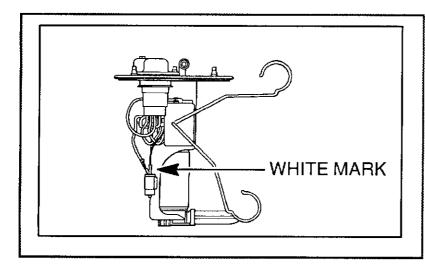
Check for normal operation of the fuel gauge sending unit. If it does not operate normally, replace the fuel tank pump and gauge assembly (listed in the PARTS INFORMATION section of this bulletin). Refer to Group 13 in the Diamante service manual.
