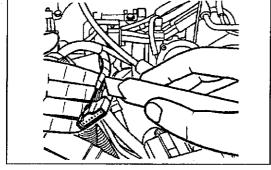
3. Use a sharp blade to open the plastic harness covering behind the main loom, to expose the wires.
