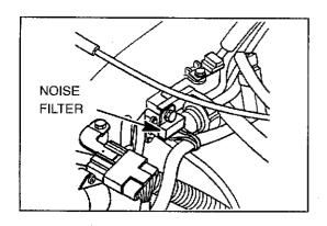
Install a noise filter (listed in the PARTS INFORMATION section of this bulletin) as shown.
