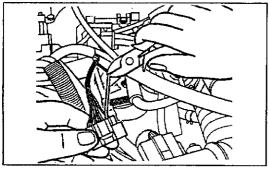
4. At pin #2, cut the white wire 2 inches from the connector.
