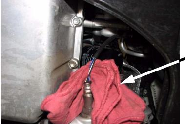
Be sure to remove shop towel after installation of new oil filter!
