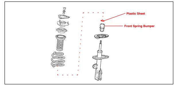
5. Reassemble the front strut assembly.
