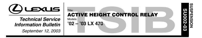
Introduction Some 2002 and 2003 model year LX 470 vehicles may exhibit a flashing AHC (Active Height Control) "OFF" light with DTC C1743 in AHC ECU memory. A change has been made to the Active Height Control Main Relay to improve relay performance.
