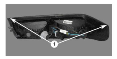
8. Install the park turn signal lamp to the vehicle by inserting the two retaining tabs (1) toward the center of the grille assembly. Then seat the park turn signal lamp outboard retaining clip by pushing the lamp assembly back into the front inner fender.
