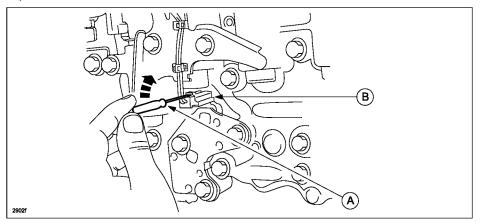
b. Remove oil pressure switch B.
