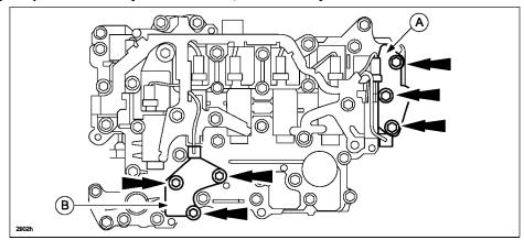
8. Connect the oil pressure switch A and oil pressure switch B connectors.
