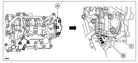
b. Remove the bolts for oil pressure switch A.
