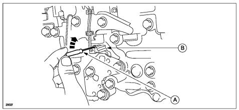
b. Remove oil pressure switch B.
