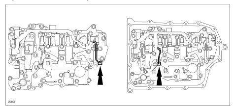
9. Install the oil strainer with new oil strainer O-rings according to the instructions on MS3 online or the Workshop Manual (section 05-17 CONTROL VALVE BODY REMOVAL/INSTALLATION [FW6AEL, FWAX-EL]).
