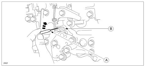
b. Remove oil pressure switch B.
