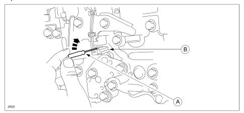
b. Remove oil pressure switch B.
