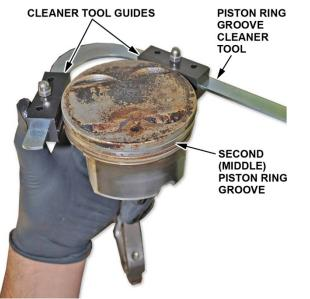
4. Press the handle on the piston ring groove cleaner tool and slide the cleaning bit onto the appropriate piston ring grooves.
