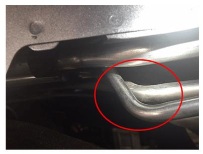
If the lines are found to be contacting each other, loosen the retaining clamps and reposition lines to gain clearance, then retighten retaining clamps.
