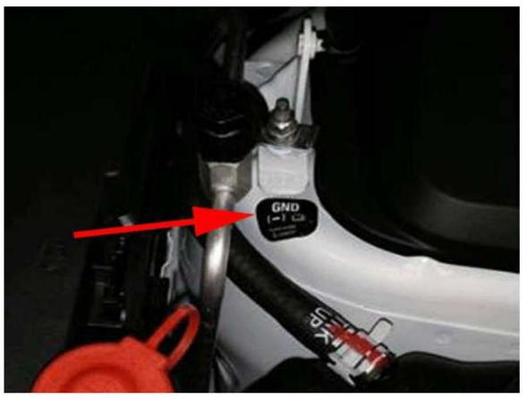
4. After fuse is replaced, install an electrical ground point label, GM P/N 10384767, in the approximate location as illustrated above.
