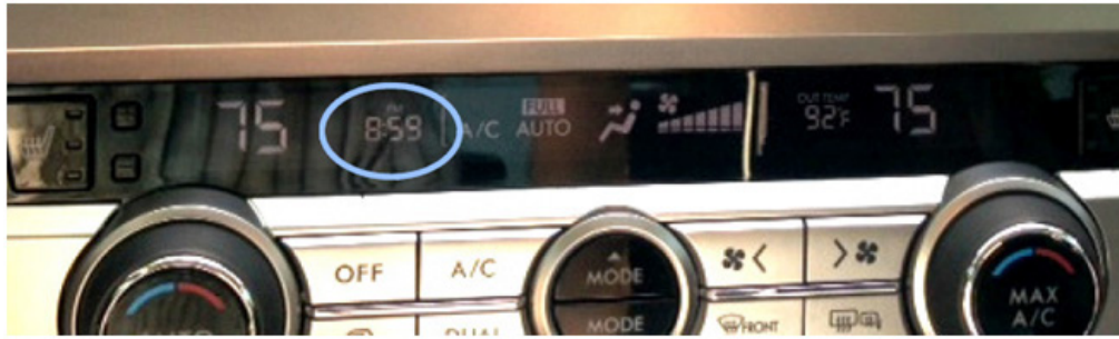
The correct time is 4:59 pm but HVAC display shows 8:59 pm.
