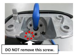
**IMPORTANT:** Avoid damaging the Phillips drive portion of the screws by using No. 2 size Phillips screw driver. They are installed with a thread locking compound and may require some extra force to remove.
