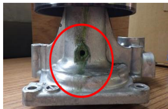
Dried coolant steam shows as green-color deposit at bleed hole.
