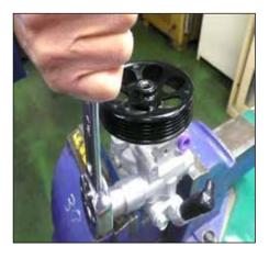
• Remove the plug using a 22mm box wrench.
