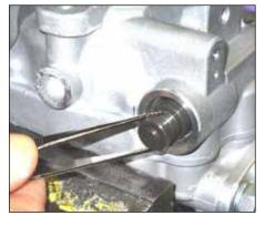
• Using a pair of tweezers, remove the relief valve. Note: Be careful not to scratch the inside of the pump housing.
