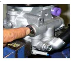
• Confirm that the relief valve moves smoothly by pushing it in and out several times.
