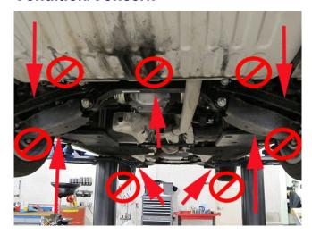
When recovering or transporting a Cadillac ATS, the under vehicle components may be damaged if the recommended towing and securing steps a not followed.
