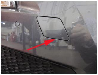
**3.2.** Carefully open the cover in the front or rear fascia by using the small notch that conceals the tow eye socket. Use care to not damaç the paint.
