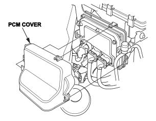
31. Remove the PCM connectors and harness clip. Remove the battery cables from the underhood fuse bo
