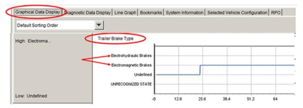
To view "Trailer Brake Control Output Circuit" 47 faults, build GDS2 as follows: CCM->Data Display -> parameter "Trailer Brake Control Output Circuit": Okay, Short to Ground, Short to Power, or Unknown. Example, shown below is a trailer with a short to ground on the trailer brake circuit.
