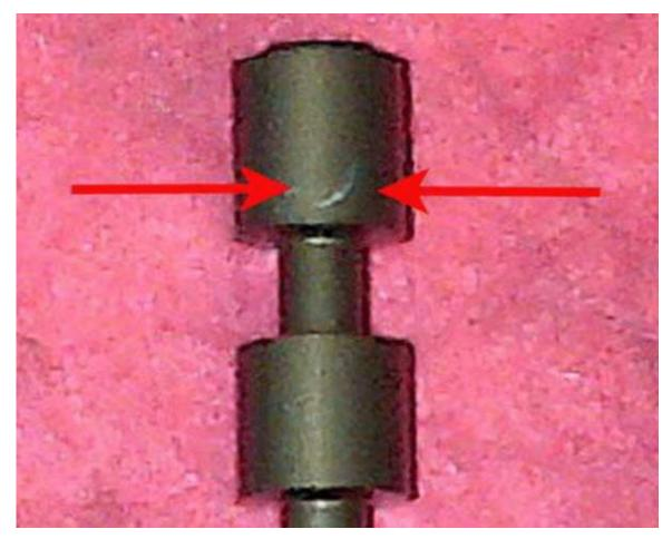
The recommended inspection procedure is to remove the valve and inspect it for any scratches on the valves. The illustration above shows an example of a valve with a scratch mark on it. If the valve is stuck in the bore or shows signs of scratching or damage, the lower valve body should be replaced.
