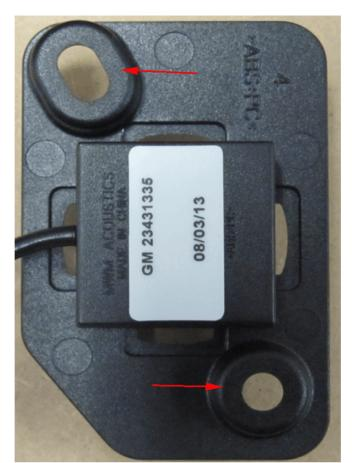
The new ANC microphone, P/N 23431335, uses screws and comes with a foam ring on the face of the microphone as shown in the illustrations above.
