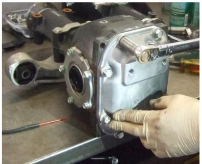
• Clean and transfer the drain plug into the new cover and install a new sealing gasket. Torque the drain plug to 60 Nm (44.3 ft. lbs.).
