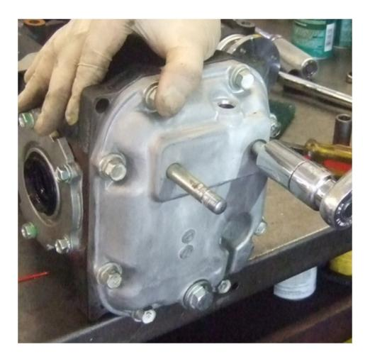
**VERY IMPORTANT:** When installing the new breather vent assembly into the rear cover, **DO NOT** tap on portion "A" shown in the illustration below. The square drive end of a 12mm ½-inch drive deep-well **impact** socket fits over and past portion "A" down onto the "flange" portion "B" and makes an excellent installation tool / driver.
