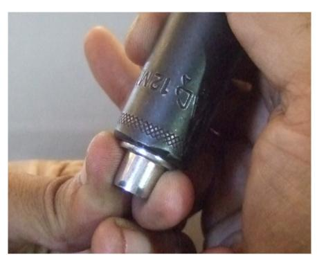
**NOTE:** The new breather vent assembly is also installed "dry" with **NO SEALER**. **CAREFULLY** tap the new breather vent into the cover while keeping the **impact** socket (installation tool) square and perpendicular as shown in the photos below. The tapping sound will change when the flange portion of the breather vent bottoms out and is fully seated (no gap) against the rear cover.
