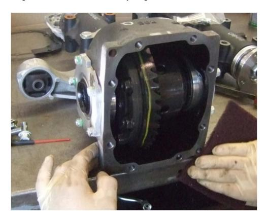
• Fit the new gasket to the cover as shown. Reinstall the 8 cover mounting bolts and torque to 44 Nm (32.5 ft. lbs). **NOTE:** The new gasket goes on "dry" with **NO SEALER**.
