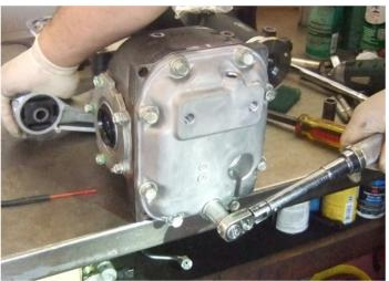
• Reinstall the 2 differential assembly mounting studs into the new cover until they bottom out. **DO NOT OVERTIGHTEN**.
