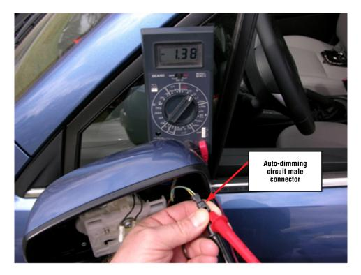
Once the Auto Dim circuit voltage is verified as acceptable, replace both exterior Auto Dim mirror glass assemblies following the procedure in the Accessory Installation Guide referenced above.
