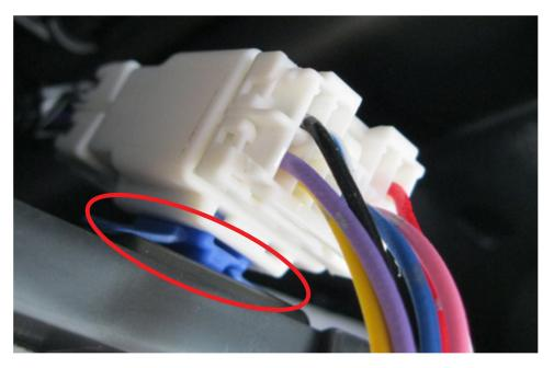
• Make sure the upper console / map light assembly's retaining claws engage above the support properly to retain the front edge **before** reattaching the 2 rear edge retaining clips and the 2 mounting screws as shown below.
