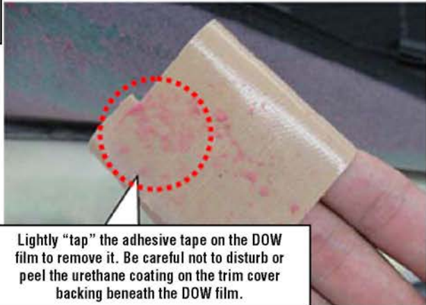
Use a piece of adhesive tape (duct or packing tape) wrapped around your fingers as shown with the adhesive to the OUTSIDE
