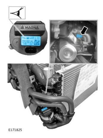
4. Install a new supercharger cooling - coolant pump (see TOPIx Workshop Manual, section 303-03).
