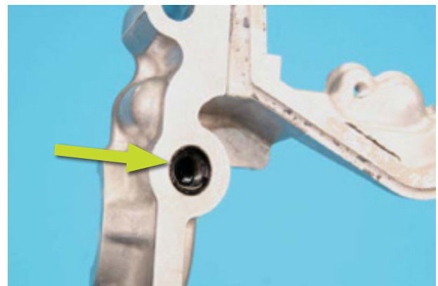
AVCS filter screens must be replaced if removed.
