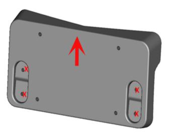
2. Install bolts through the license plate bracket and fascia holes.
